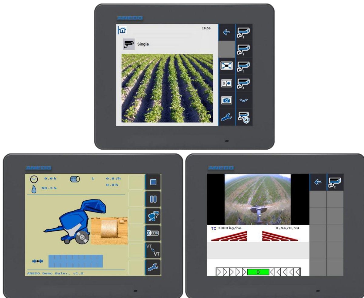
Fig. 1: Current panel apps with digital video support; Cam-Digi (top), UT (bottom left) and Layout Manager (bottom right)
